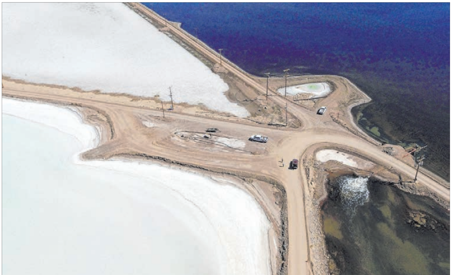
Brine evaporation ponds at Albemarle's lithium mine Sept. 21 in Silver Peak. It is still the only lithium producer in the U.S.
